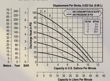
NOTE: Performance based on the following: elastomeric fitted pump, flooded suction, water at ambient conditions. The use of other materials and varying hydraulic conditions may result in deviations in excess of 5%.
