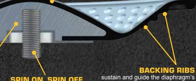
**OVERSIZED INTEGRATED PLATE** supports nearly 50% of the diaphragm through the entire dynamic motion stroke.
