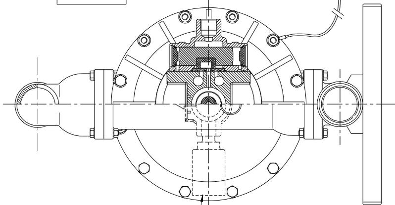
Sectional General Assembly :- B50 / X50 Full Flow 2:1 Metallic Pump
