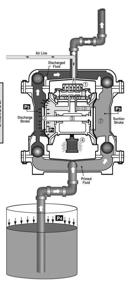
Air-Operated Double Diaphragm (AODD) pumps are powered by compressed air or nitrogen.
