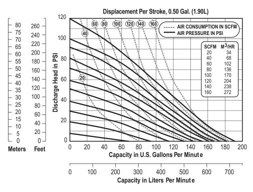
NOTE:For U2 pumps fitted with PTFE diaphragms, reduce water discharge figures by 20%. Suction lift is reduced to 10' (3.05m) dry and 20' (6.10m) wet.
